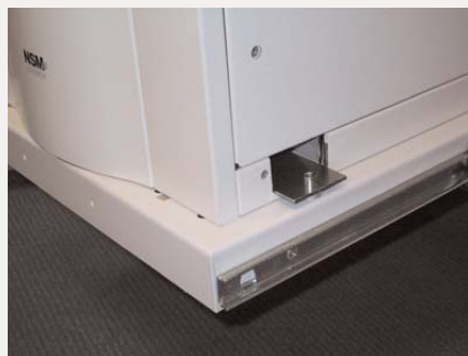
Mounting hardware secures the library to the bottom of the retractable platform.
