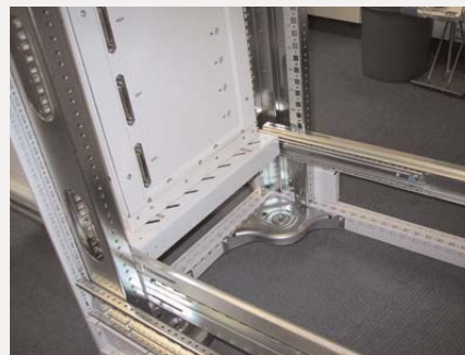
Rolling guides allow quick and easy service access to the sides and rear of the library.
